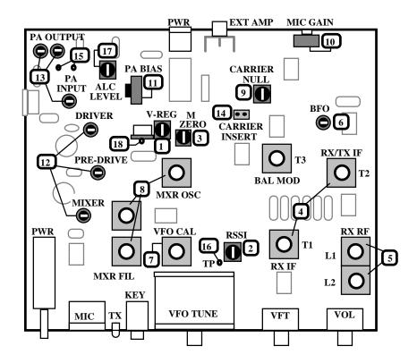
**Note:** For trimpots, trimcaps, and IF cans (T1-T3), use a non-conductive tuning wand with a metallic tip. For TOKO brand inductors, use a non-conductive wand with a narrow plastic tip. For Coilcraft brand inductors, use a small hex-head non-metallic tuning tool.
